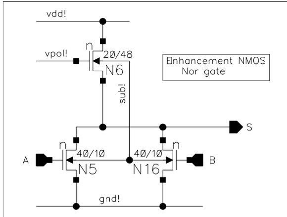
figure 3 : NOR schematic
